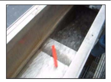
Figure 1 - A PTAGIS diagnostic test (stick) tag activating a typical slide gate.
