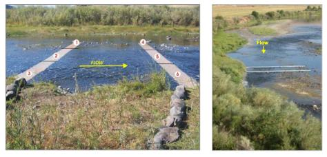
Figure 3. Photos showing the six antennas in the two 3-antenna array configuration
